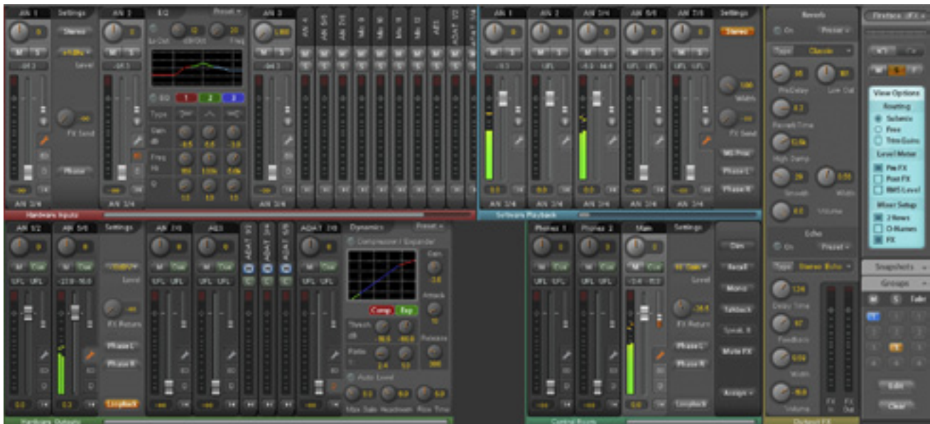
Each Hardware Output channel (bottom row) is like an analogue mixer's bus returns. Rather than cluttering the upper channels' rows with send controls, the parameters of the Hardware Inputs and Software Outputs can be tweaked, including the new EQ, Dynamics and Reverb/Echo settings. Monitor mixes can be auditioned via a pre-defined Master Control Room output using the Cue buttons.
